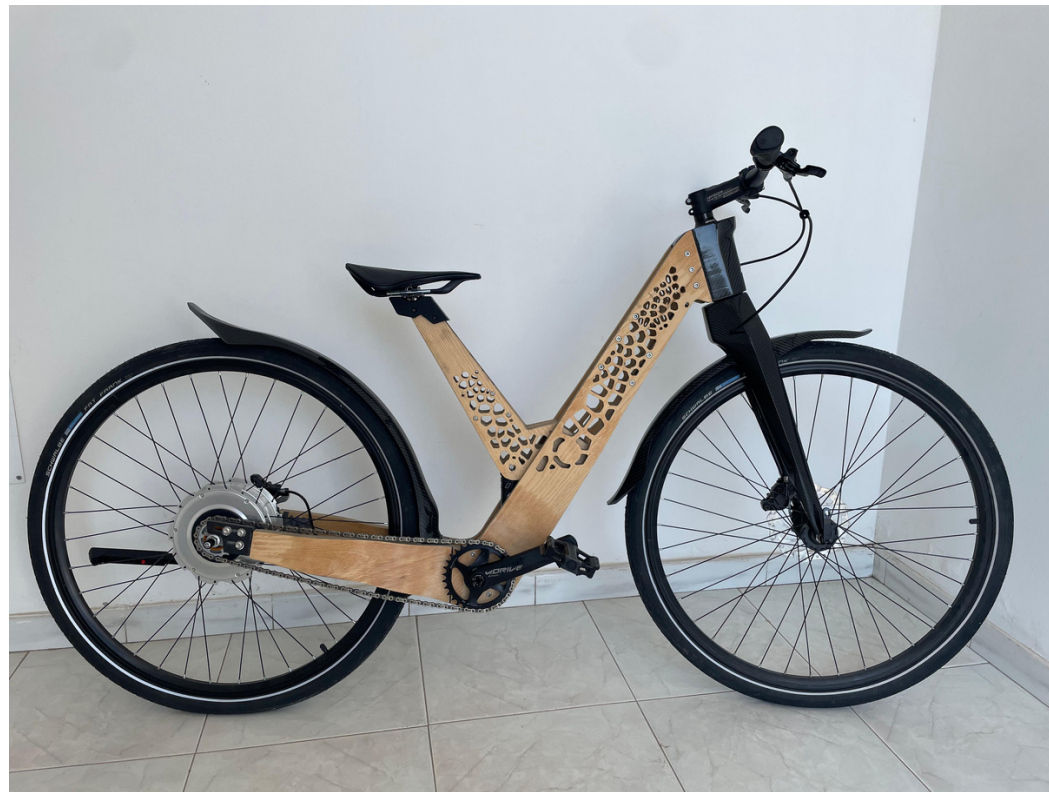
Bike prototype made of plywood and recycled carbon!
